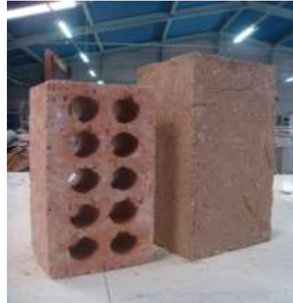
Figure.4 Laboratory-produced unfired brick compared with fired brick
