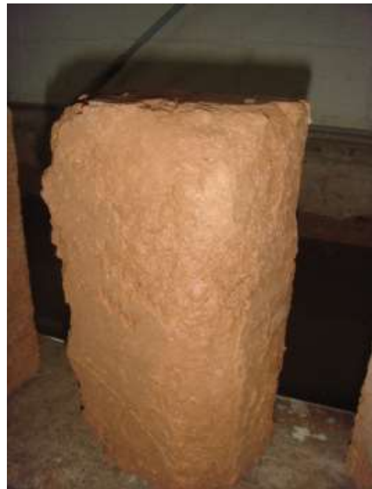
Figure (9): Appearance of brick after saturation test
