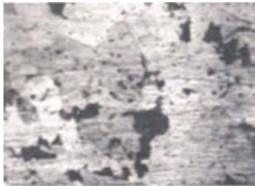
Sample No. 6 Annealing Temperature 920 °C, 5 min. period
